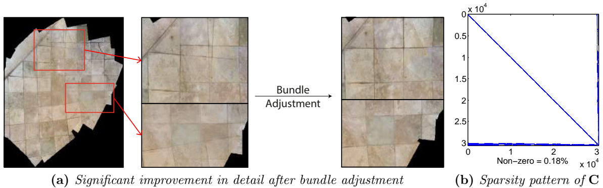
FIGURE 2.15: The algorithm produces visually pleasing results when making granular refinements in feature-dense scenarios. The above example shows a mosaic of 54 photos with 30,542 unknown parameters ( \mathbf{X} \in \mathbb{R}^{30542} ). Before, there are large errors due to perspective distortion and drift. The algorithm adjusts global feature positions \hat{\mathbf{f}}_i and image transformations \mathbf{H}^j jointly to minimise the objective function. \mathbf{C} (right) forms an “arrowhead” matrix, such that individual features lie along the top-left 2n \times 2n block diagonal and are coupled to images in the last 8m rows/columns if their corresponding elements are non-zero.
